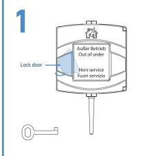
To open the MCP, rotate the lock door counterclockwise and use the supplied key
