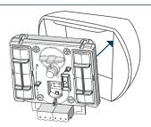
Install the sounder interface module into the base locating the bottom tags and pushing back in.
