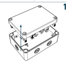
Remove the lid from the back box, removing the screws on the corners.
