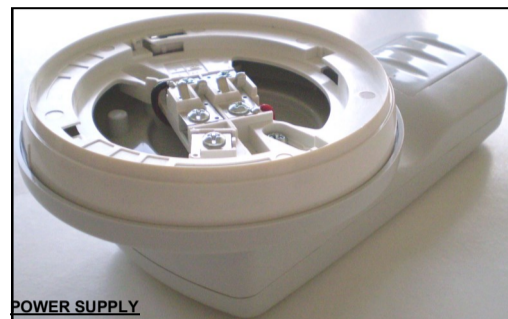
Picture 2 - the adaptor base for sensors on the programming unit
