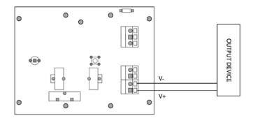
Wiring example for the relay switch output.
