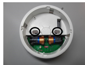
Picture 8 - position of the holes for screw's insertion
