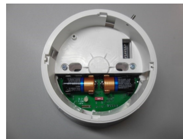
Picture 6 - primary and secondary batteries inserted
