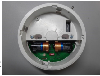
Picture 2 - wireless base sounder top view
