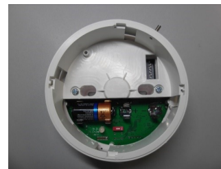
Picture 5 - secondary battery inserted
