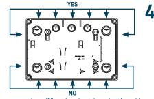
Prepare apertures (20mm knockouts) required for cable access and fit appropriate rated glands.
