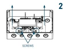
Remove the electronic PCB assembly from the enclosure. The PCB is held by two Philips screws below the display, it then slides up and out.
