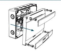
Remove top and bottom front plastics that cover screws, unscrew all four screws and remove the lid from the back box.
