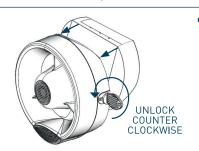
Remove the mounting from the sounder by inserting the security key and turning to the unlocked position on both sides. Pull apart the two pieces.
