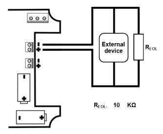
Wiring example for the relay switch output.
