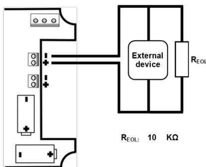
Wiring example for the relay switch output.
