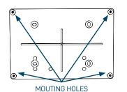
Using a suitable-sized drill bit (4mm) drill the pre-defined screw mounting points in the 4 corners of the backbox.
