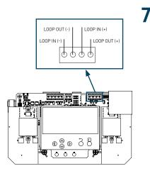
The Loop connector on the top of the translator board should be wired to the Panel of your choice, from the left to right the terminals are:
