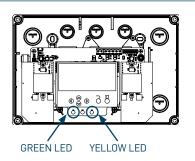
Ensure the LED indicates that the discovery mode is enabled, alternating green and yellow colors.
