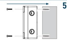
Screw the back box to the wall using all fixing holes and appropriate-sized roundhead screws (do not use countersunk screws).
