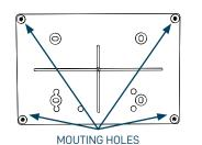
Using a suitable-sized drill bit (4mm) drill the pre-defined screw mounting points in the 4 corners of the backbox.
