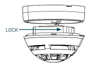
• Ensure you replace the battery cover as this forms part of the detectors anti tamper protection and refit the detector locating it into the base twisting clockwise.
