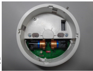
Picture 2 - wireless base sounder top view
