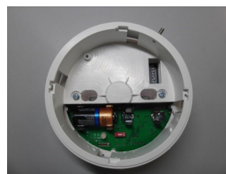
Picture 5 - secondary battery inserted
