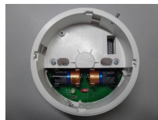
Picture 6 - primary and secondary batteries inserted
